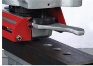
Punching Channel Flangers And Angles
